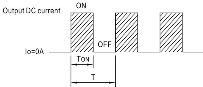
$$\text{Duty cycle(\%)} = \frac{T_{ON}}{T} \times 100\%$$
